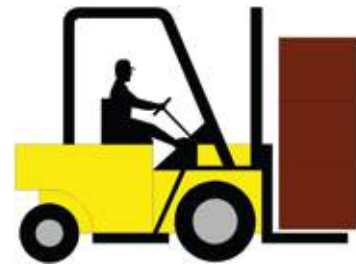
Figure 11: Use forklift for loading, unloading and storing of a circuit breaker
